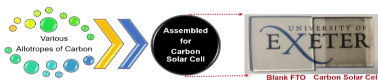
Figure 1. Digital image of the carbon solar cell as fabricated by solution-processed layer deposition of different allotropes of carbon (as a single source).
