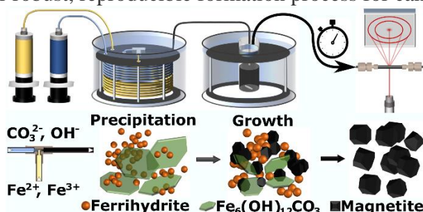
Figure 1. Schematic of the set-up for nanoparticle synthesis showing the syringe pumps used to feed reactants to a T-mixer, pre-heated water bath, and aging bath; and the synchrotron X-ray diffraction set-up showing the solution injected into a quartz capillary for analysis.
